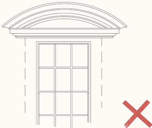
Incorrect proportions of arch/lintel to window opening
